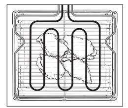
For grilling thin cuts and for browning food. The inner part of the upper heating element gets hot.
